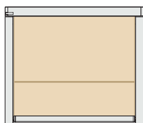
Transverse seam in the bottom third (standard, no surcharge)
