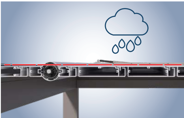
Louvre positioning when it rains
