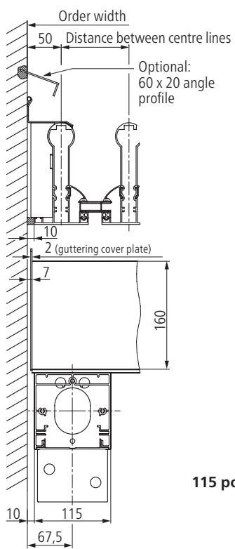
Gutter and post position on the wall
