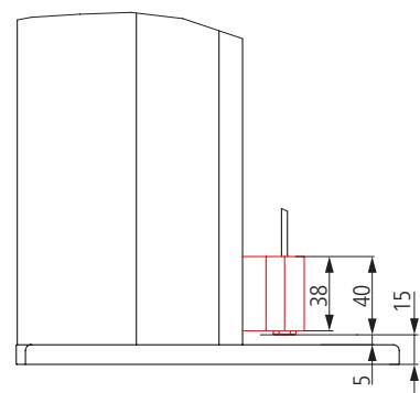
115 post with 20 x 38 x 28 mm rope holder (is used with the "outside rope guide" version)
