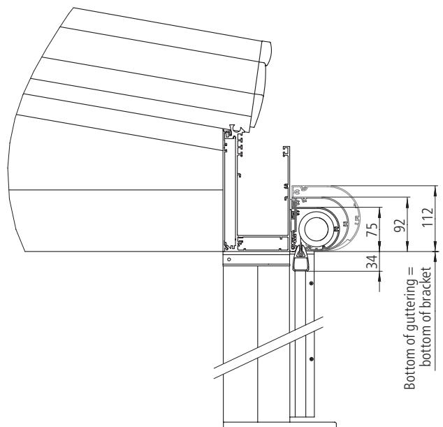
220 guttering with side bottom lateral locking bar
