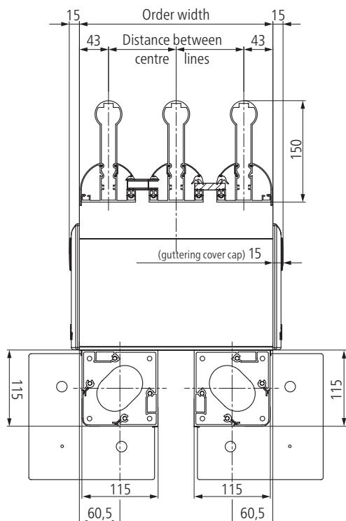
Gutter and post position on the wall
