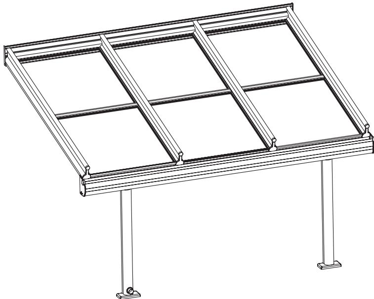
If the outer posts are indented, the centre post can be omitted for certain roof dimensions. Additional steel reinforcement bars in the guttering or the crossbeam also permit the number of posts and spacings to be changed.
