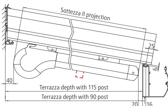
The sun protection runs below the roof support. Combined with LED light bars or LED Design, the Sottezza II must be mounted using suitable spacers at a spacing of 30 mm to the roof supports.
