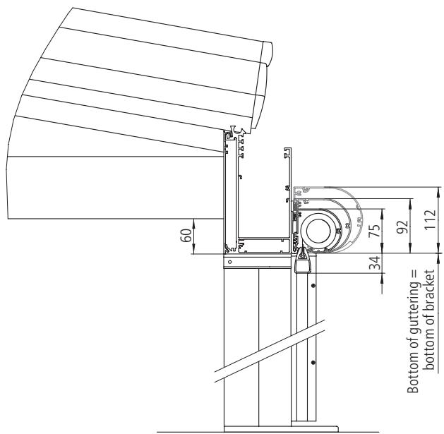
220 guttering with side top lateral locking bar
