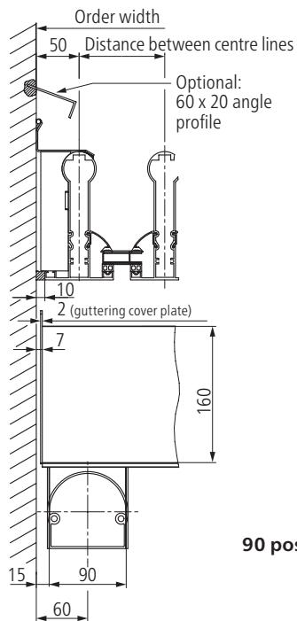
Gutter and post position on the wall
