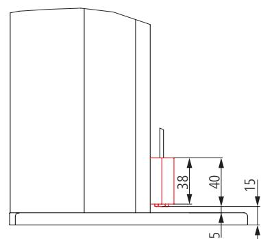
115 post with 14 x 35 x 16 mm rope holder (is used with the "indented rope" version)
