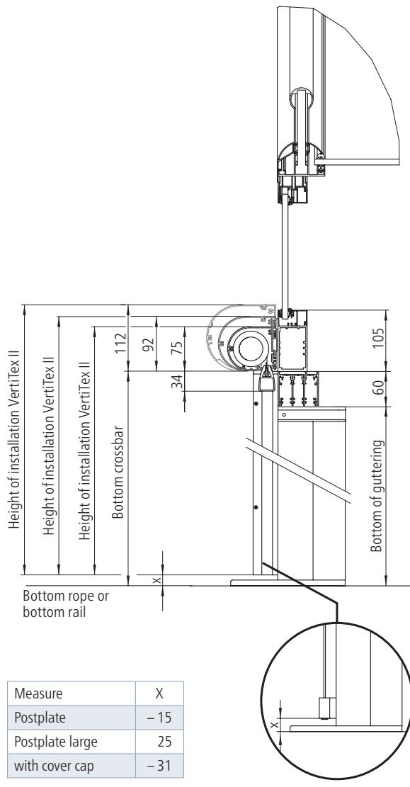
220 guttering with side top lateral locking bar
