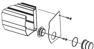
Drain on the side of the 160 and 220 guttering incl.
