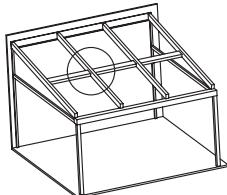
From a pane length of 3,000 mm, it is advisable to split the roof glazing by means of a rigid transom.
