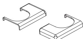
Cover cap for post plate wall left/wall right
