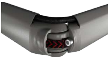
7) bionic tendon and hidden cable conduits in the arms
