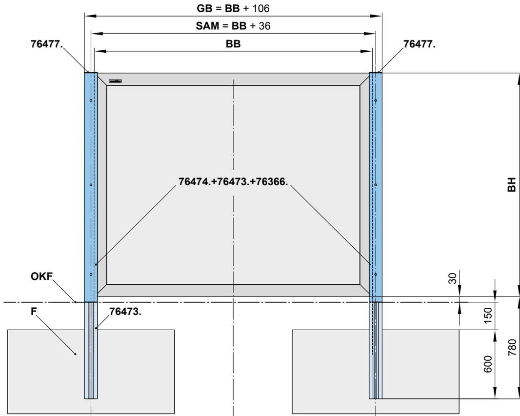
The structural design of the posts was based on a stagnation wind pressure of 585 N/m<sup>2</sup>, wind load zone 2, mixed profile 2 and 3 (inland). This corresponds to wind speeds ranging from 24.5–28.4 m/s, wind force Beaufort 10. When calculating footing sizes, local idiosyncracies (wind load zone, terrain category, etc.) need to be taken into consideration.
