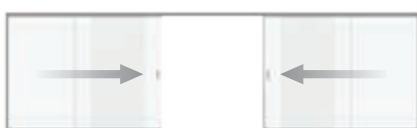
Lockplate version – opens on two sides, closes in the centre
