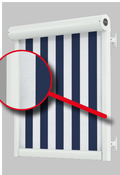
units with the optional tracfix system have no annoying gap between the cover and the guide track. When completely extended the front profile finishes flush with the end of the guide tracks
